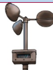
An anemometer measures how fast the wind is blowing.
